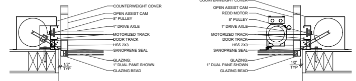
01 DOOR JAMB MOTORIZED SCALE: 1-1/2" = 1'
