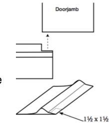
threshold. Seat the notches of the threshold on the interior corners of the doorjambs, and operate the door to make sure the bottom seal and the hump on the threshold make good contact without inhibiting the door's movement.
