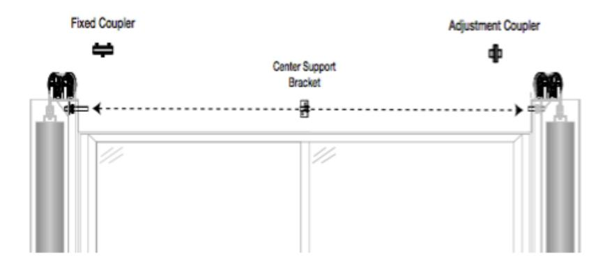
C. After you align the cam pins, apply a thread-locking compound to the adjustment screws on the adjustment coupler, and tighten them.
