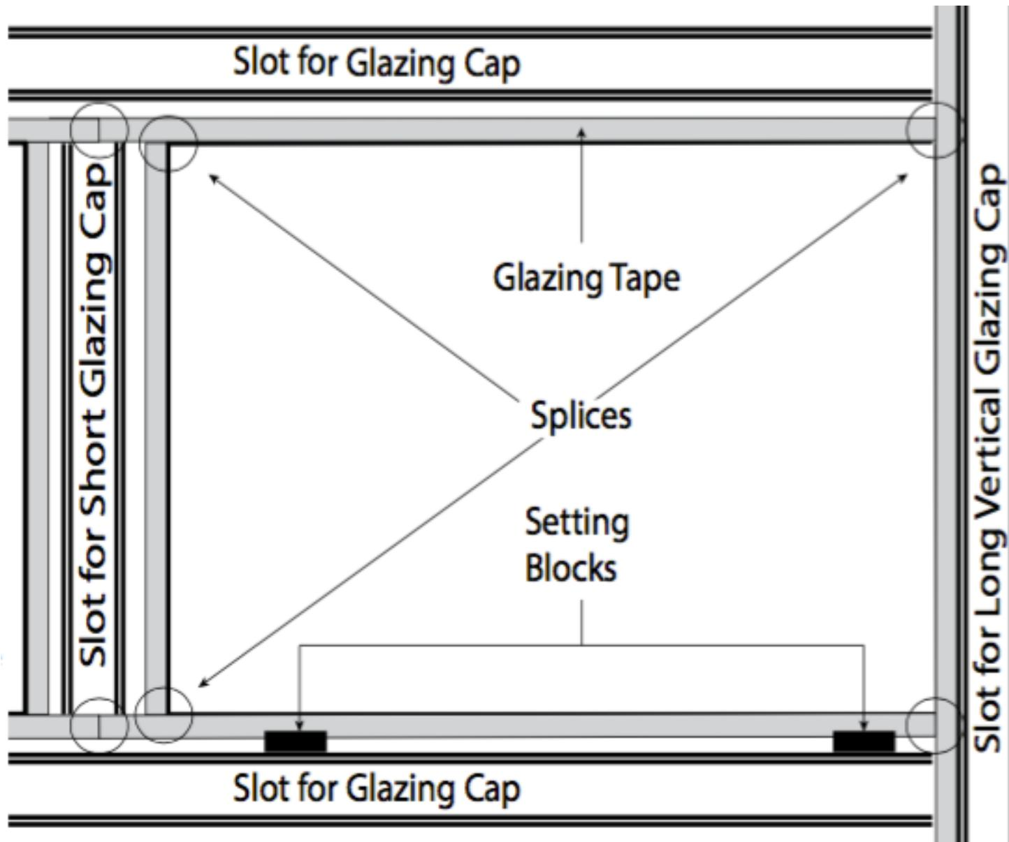
D. Apply the sealant in the shipment (Dow Corning 995 Sealant) to every splice in the tape, and place a setting block where each corner of the glass panels will sit.
