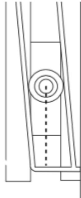
B. Then rotate the adjustment coupler to move its trolley up or down so that its cam pin is aligned with the other one.
