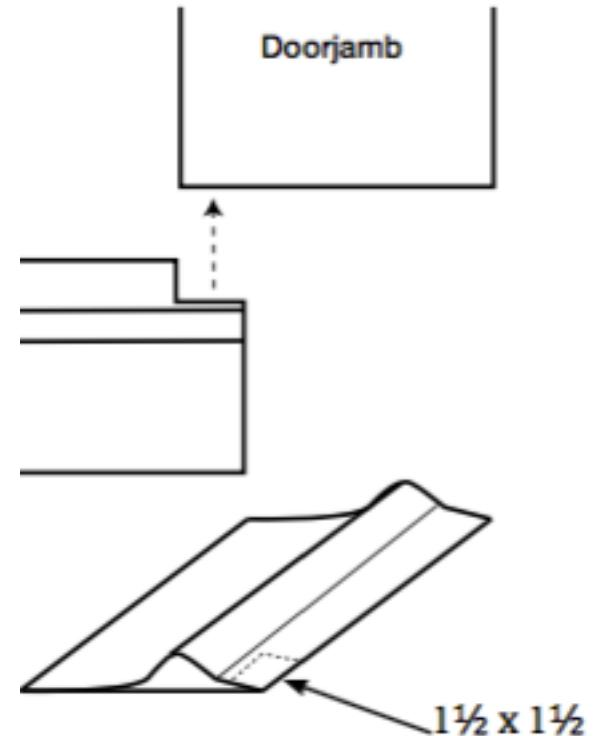
D. Drill pilot holes in the floor for the screws through each of the predrilled holes in the threshold. Move the threshold, and apply a bead of structural adhesive that is 5/16 of an inch thick between the pilot holes where the threshold will lie.
