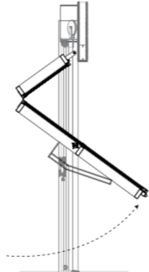
Close the door by gently pulling the bottom down until the door closes fully.
