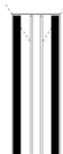
C. Cut the seals of the outer caps flush at the caps' ends. (See the thick dotted line in the illustration below.)
