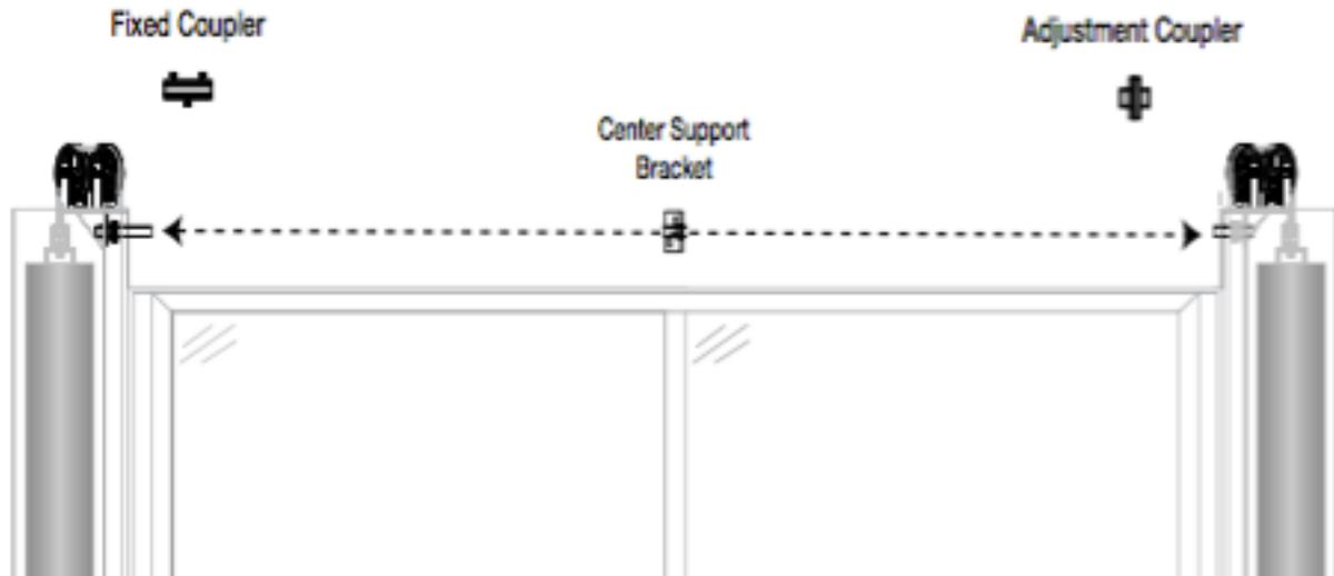
D. Install the adjustment coupler on the same side as the motor so that you do not have to move a ladder back and forth when you align the cam pins; and only slightly tighten the adjustment coupler because you will need to turn it by hand when you align the cam pins.
