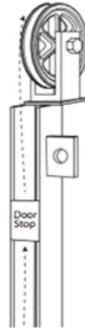
B. If you are installing a set of doors that will share a counterweight, route the shared cable for one door, and after you have fastened its operating channels, route the cable for the second door. The cable will be draped between them for you to hang the counterweight from its center.
