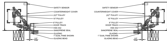
03 DOOR JAMB NON-MOTORIZED SCALE: 1-1/2" = 1'
