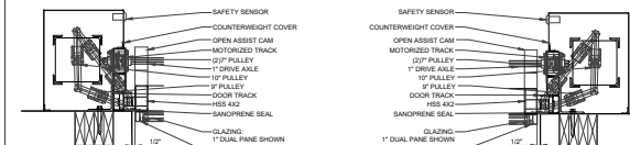
01 DOOR JAMB MOTORIZED SCALE: 1-1/2" = 1'
