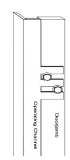
For wooden doorjambsInstall the lag screws from the shipment according to this illustration; we will send washers in the shipment if the lag screws need them.
