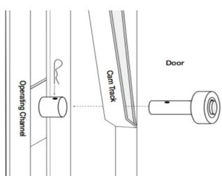
C. Insert the cam pin into the pin sleeve, and secure it with the cotter pin.
