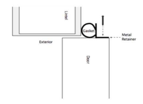
retainer, and screw the retainer into illustration. Make sure no light.
