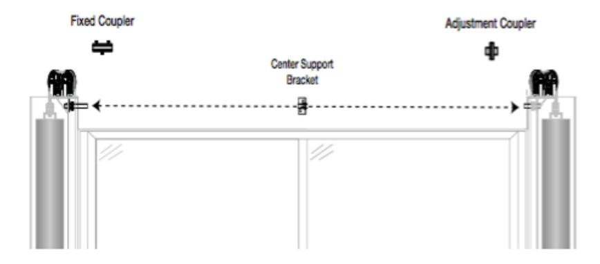
C. After you align the cam pins, apply a thread-locking compound to the adjustment screws on the adjustment coupler, and tighten them.
