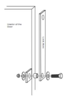
\* CAUTION: The threaded ends of the bolts must always protrude on the door's side of the lug, rather than the channel's side, so that they don't rub the cables.
