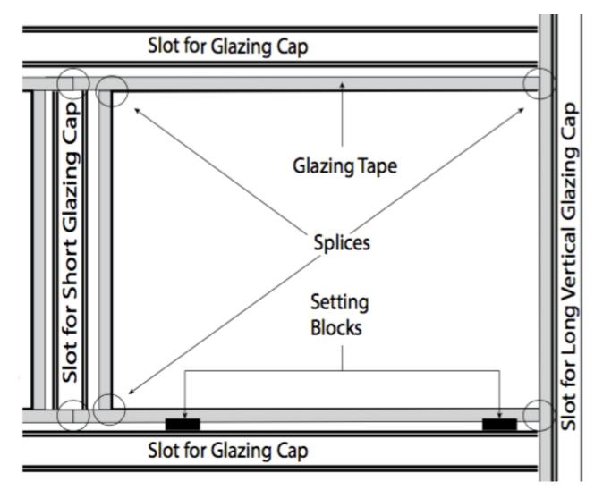
Process 4-Installing Glass (For doors with
