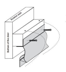
B. The drip edge of the gasket should face the exterior side.
