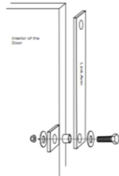
C. Always use an open or box wrench, never an adjustable one, to tighten the nuts and bolts. Do not tighten the bolts excessively.
